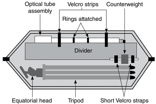
When placing a tube assembly into the case, it may be necessary to remove certain accessories, such as the finder scope or diagonal and eyepiece assembly, to ensure a proper fit. Try it first with the accessories attached and see if the case can be zipped up easily. If the fit is too tight, remove accessories as needed and store them inside the case or in the outside accessory pocket (available on some cases).
